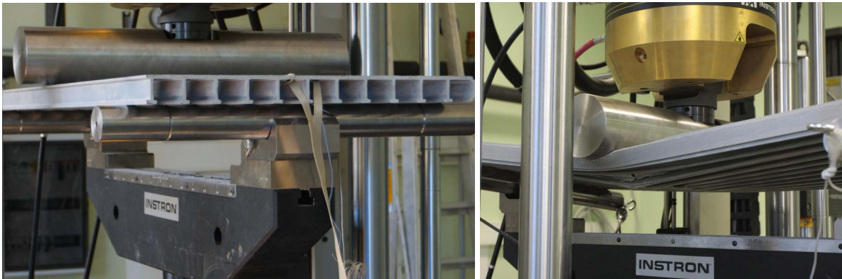
Figure 3. The experimental three-point bending test setup and collapse mode of the stiffened deck structure
